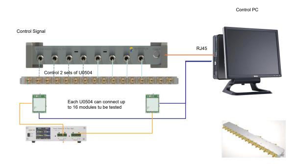
\*The Sunyield RF switch matrix U0504.can realize 1 to 4 mapping of RF signals, and map the SX-7500 RF port to a maximum of 32 signals.
